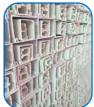
smaller trunking insert into bigger one
